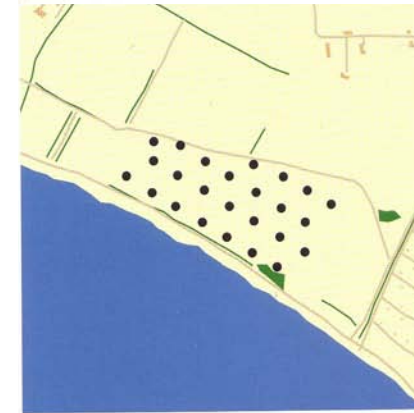
25. Thyholm, 20 Vestas/Bonus lattice tower turbines, 55 kW, 1985, hub: 22 m, dia: 16 m. Main structure: rows interplay with power poles and infrastructure.
