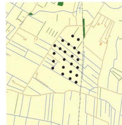
1. Avedøre, 12 Bonus tube tower turbines, 300 kW, 1992-93, hub: 33.5 m, dia: 31 m. Follows the coastline, connected to Avedøre power station, industrial technical features.
