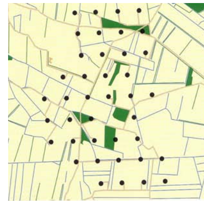
19. Rejsby, 40 Micon tube tower turbines, 600 kW, 1995, hub: 45 m, dia: 38 m. DK's most recent & most powerful wind farm, tight quadratic network, independent of roads and vegetation, flat terrain.
