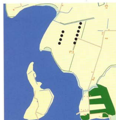
17. Oddesund, 25 Bonus tripod wind turbines, 95 kW, 1985-86, hub: 24 m, dia: 19.4 m. Broken row system, railway and high-tension transmission line.
